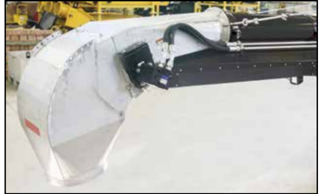
Fig 4 - Discharge with hydraulic motor
