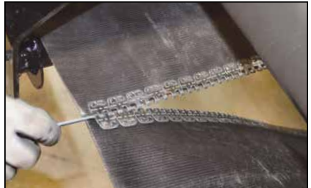
Fig 20 - Thread lacing cable
