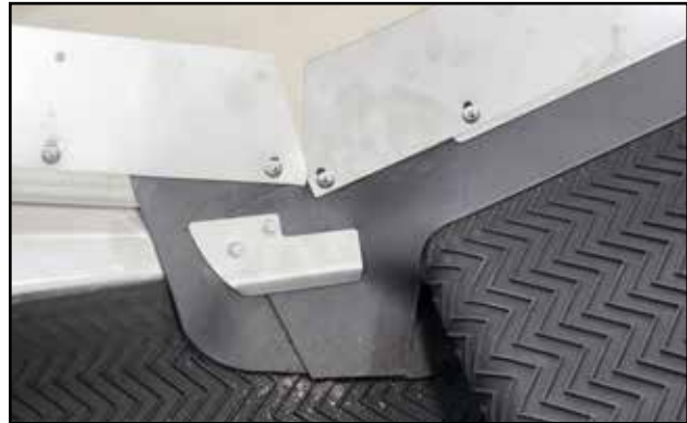
Fig 31 - Fasten flashing clamp
