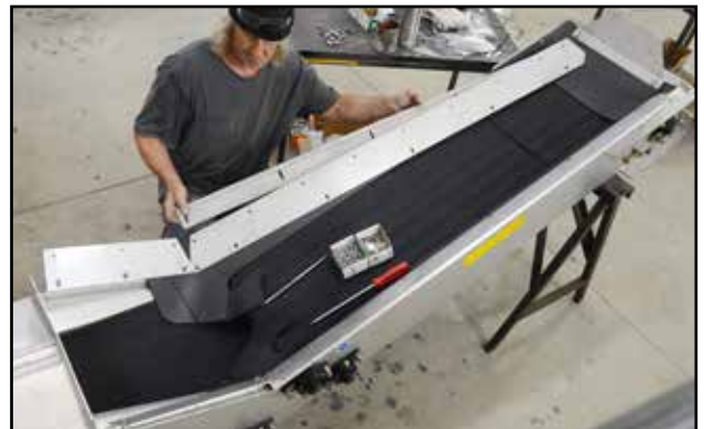
Fig 28 - Side panel and hold-down plate
