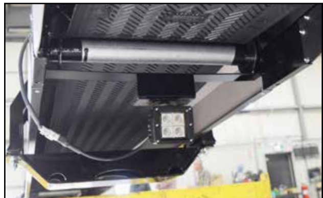
Fig 11 - Discharge work light
