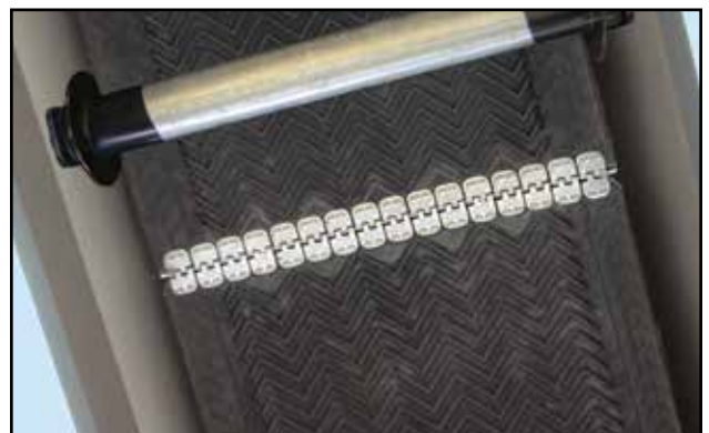
Fig 7 - Skived chevron belt with Alligator® lacing
