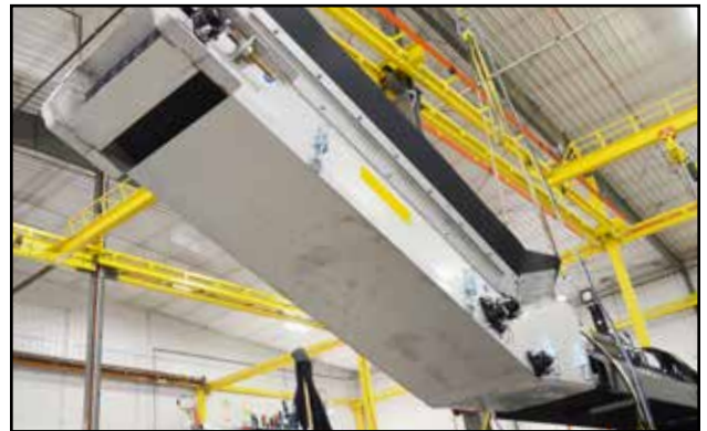
Fig 13 - Hopper Containment Assemblies
