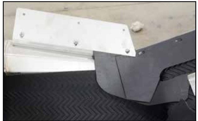
Fig 27 - Transition flashing and panel
