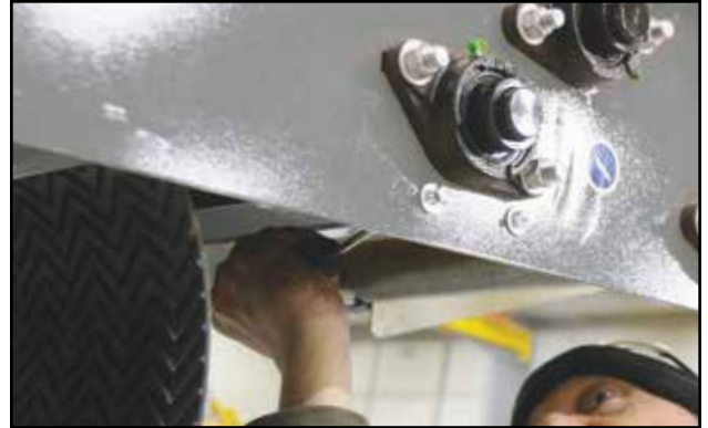
Fig 19 - Reinstall the containment plate
