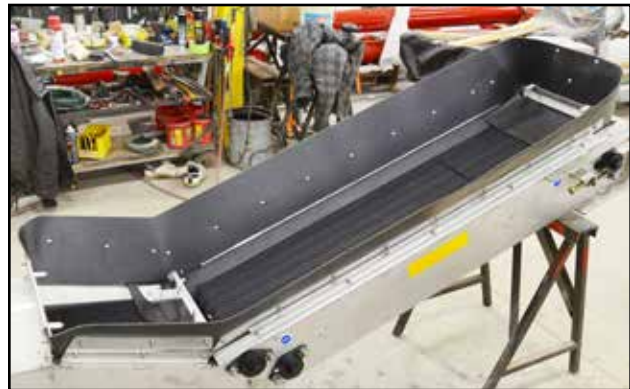
Fig 32 - Rubber belting installed
